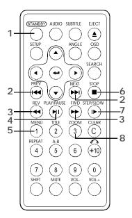
1 STANDBY button Press this button to turn on or enter standby mode.
